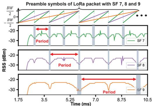
Figure 2. Detailed RSS evolution after reaching a steady value. Depending on the employed SF, one can observe a different periodicity and amplitude of the RSS profile.
