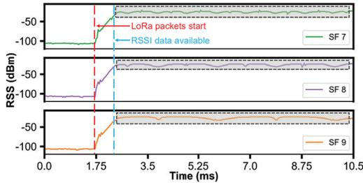
Figure 1. RSS values recorded by a LoRa device when receiving the preamble of packets sent using different SFs.
