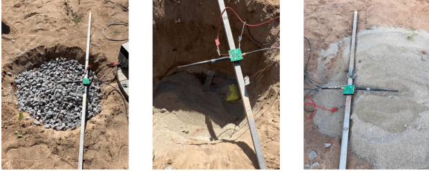
Figure 3: Experimental setup: a 60 cm deep hole that we gradually fill with different materials, such as sand, stones of different sizes, and earth.
