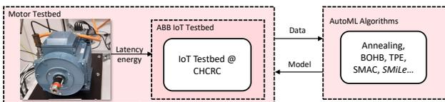
Figure 1: System overview - motor testbed and AutoML based design space exploration
