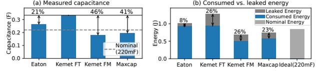
Figure 2: Measured capacitance (a) and energy leakage (b).
