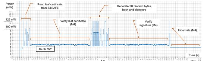
**Figure 2. Power consumption for STM32WL55JC (M4) to perform authentication with the aid of STSAFE-A110**
