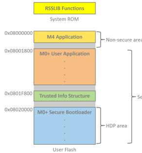
**Figure 1. Flash partition and applied secure areas.**
