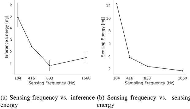
Figure 13: Impact of sensing frequency on inference and sensing energy at a fixed window size of 300 samples
