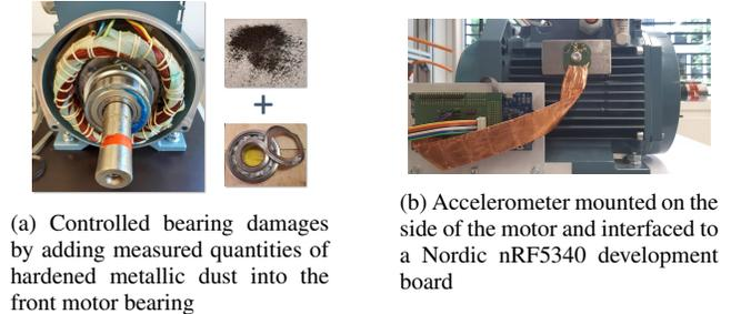
Figure 2: Motor bearing fault prediction setup
