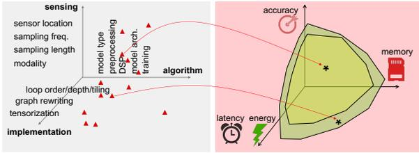
Figure 1: Challenges for edge analytics - (i) enormous design space covering sensing, machine learning and implementation, (ii) design constraints relating to latency, memory, energy consumption, and their complex trade-offs
