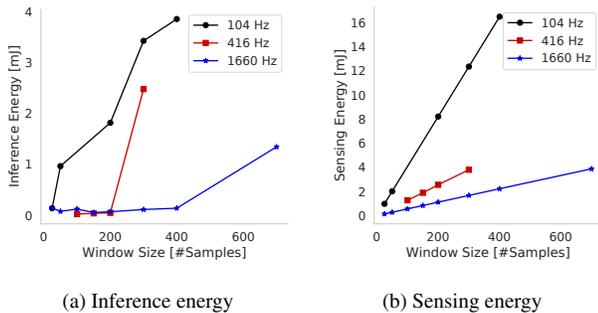
Figure 12: Impact of window size on inference and sensing energy consumption at different sensing frequencies
