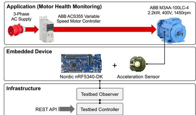
Figure 6: Architecture of a motor testbed used to evaluate *SMiLe* for the purpose of motor bearing health analysis
