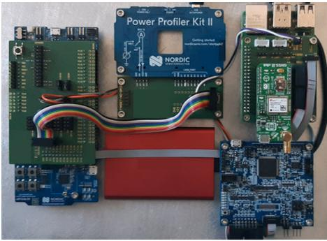
Figure 7: Testbed observer based on a Raspberry Pi4 interfaced to commercial power profiler, JTAG programmer and a Nordic nRF5340 development kit
