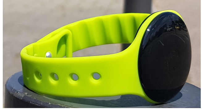
Figure 5. The TB prototype used in trials features a low-power nRF52840 SoC with additional 2 MB storage. With costs below 10€, it enables low-cost participation in the contact-tracing process. Designed as a wristband, the circular core can also be used as a key fob or a necklace. Picture by Benjamin Walczak.
