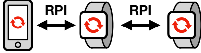
Figure 1. The low-cost TraceBand (TB) integrates seamlessly into the Exposure Notification protocol by Apple and Google, exchanging rolling proximity identifiers (RPIs) as pseudonyms with smartphones and other TB devices. The release of identifiers upon an infection allows others to identify risk contacts.
