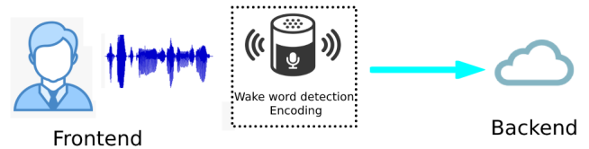
Figure 1. Personal Voice Assistant (PVA) system overview. The device (front end) is activated by recognising a wake word (e.g. 'Alexa'). The sound recorded after the wake word is transported to a back end for further analysis (e.g. Automated Speech Recognition (ASR))
